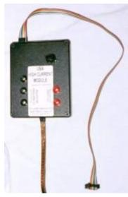
This module allows discharging a battery at up to 15 Amperes (or 50A with the Very High Current Discharge Module). It works in conjunction with a load that you supply and a UBA4. It connects and disconnects the load while measuring the load current. For the load, you can use automotive lamps, power resistors or even an active load.
