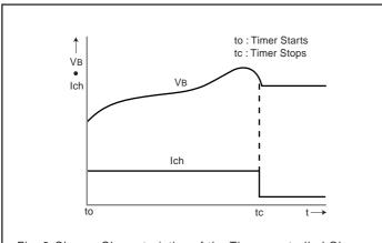
Fig. 3 Charge Characteristics of the Timer-controlled Charge System
