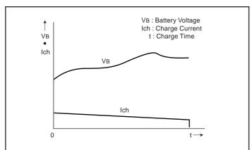
Fig. 1 Charge Characteristics of the Semi-constant-current Charge System
