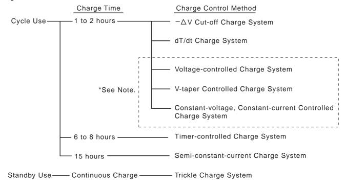
\* Not a recommended charge method for Ni-Cd batteries
