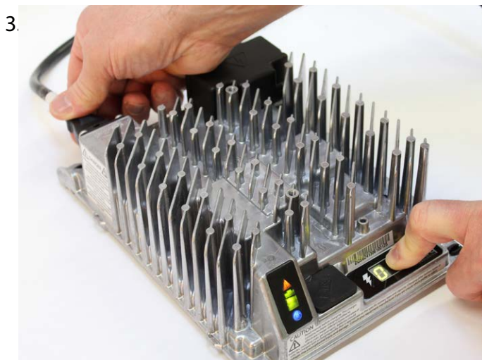
Figure 29. Reconnect AC input while holding the Select Charge Profile Button.
