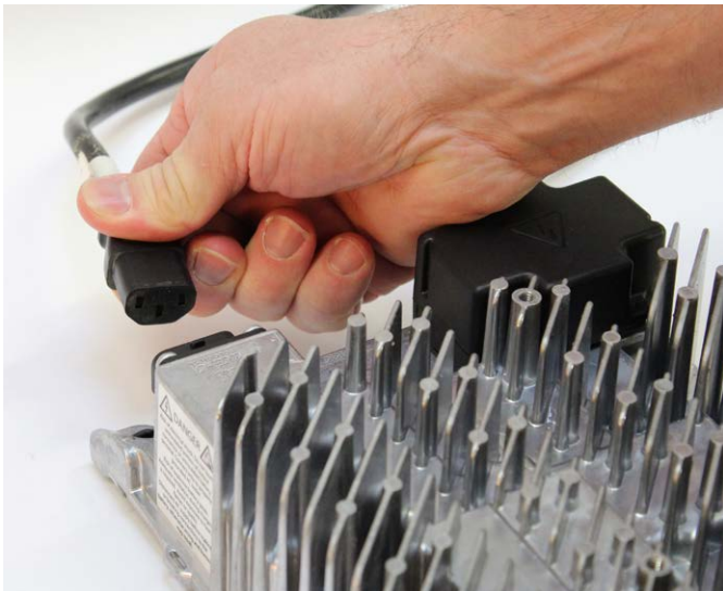
Figure 28. Disconnect AC input from the charger.
