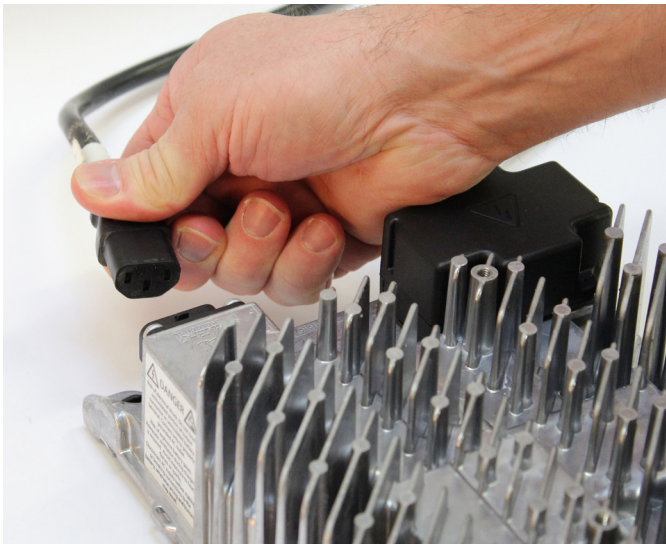
Figure 1. Disconnect AC input from the charger.
