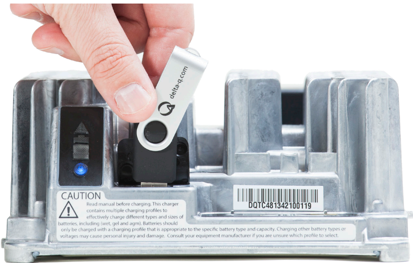
Figure 4. Insert the USB flash drive to begin the reprogramming process. When complete, the Fault / Error / USB indicator will be solid green as shown.
