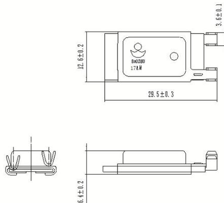
注 note: 材料耐温 Temperature resistance of materials  $180^{\circ}\text{C}$
