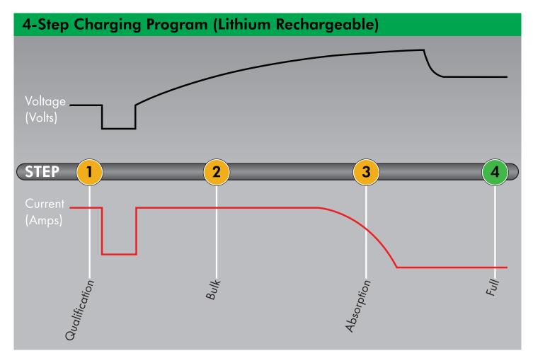
QUALIFICATION Battery condition is checked prior to charge or recovery. Charge will not be initiated if
