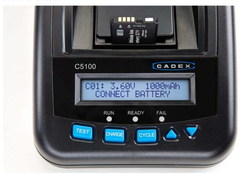
Test Performs battery rapid test using Cadex
