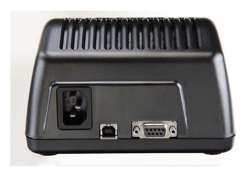
Serial port To connect to a computer. Cable not
