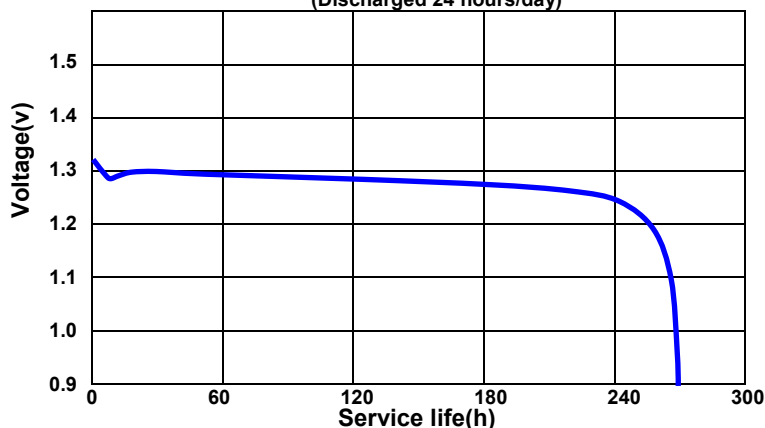
DISCHARGE CHARACTERISTICS AT 620Ω 20°C 60%RH (Discharged 24 hours/day)
