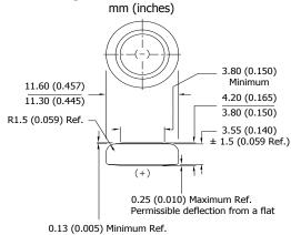
(applies to top edge of gasket or edge of crimp, whicever is higher)
