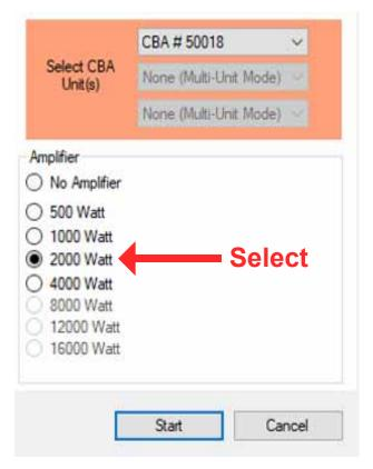
Tip: Leave the amplifier in-line, but switched off, and de-selected in the software, for discharge rates less than 100 watts (An amplifier is bypassed and disabled whenever it is powered off).
