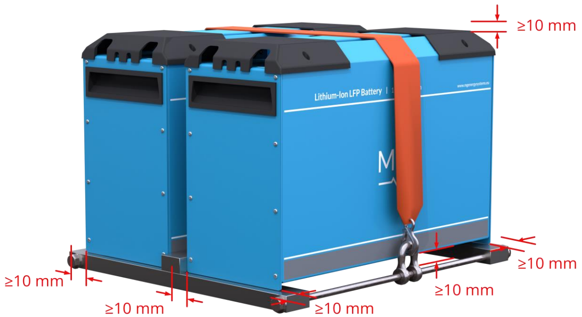
Figure 9 - Battery spacing requirements
