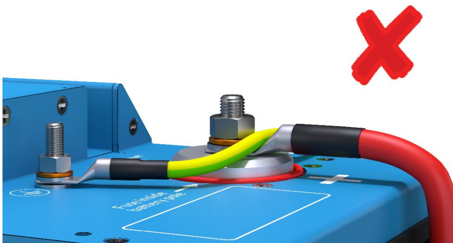
Figure 15 - Wrong routing of equipotential bonding wire
