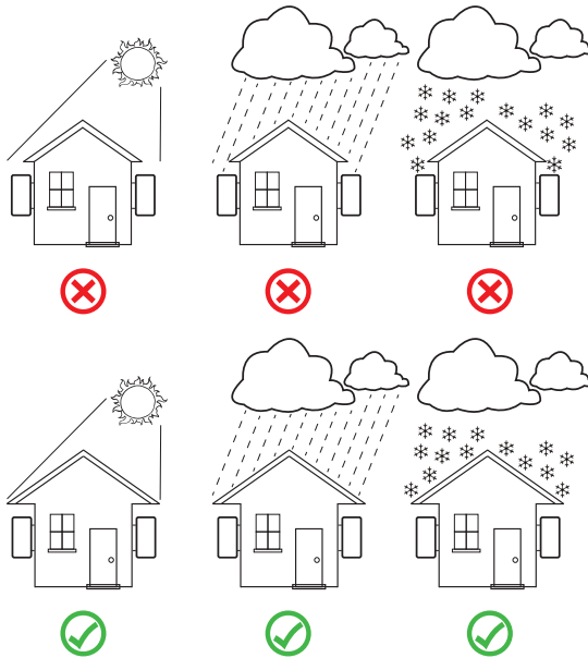
Pic 4.1 Recommended installation place
