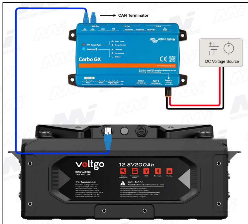
Figure 3: Voltgo Battery to Cerbo GX Connection via BMS-CAN Port.
