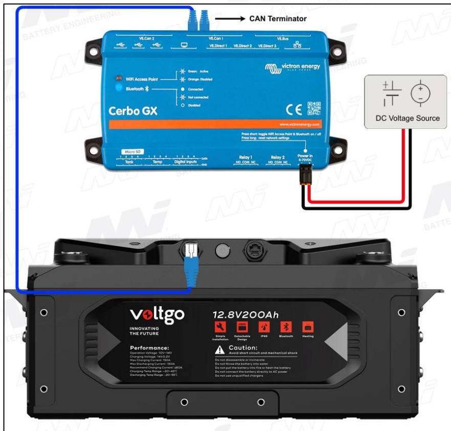
Figure 4: Voltgo Battery to Cerbo GX Connection via VE.CAN Port.
