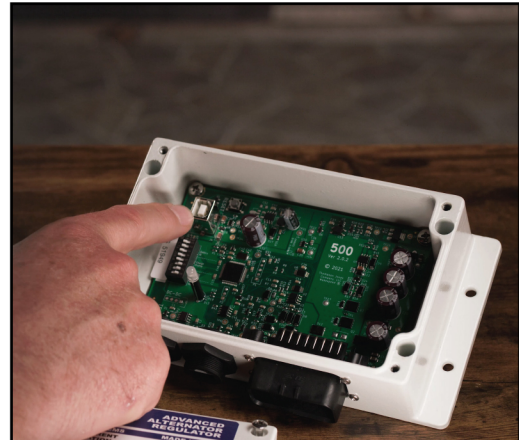
Figure 5 - Type B USB connector & reset button
