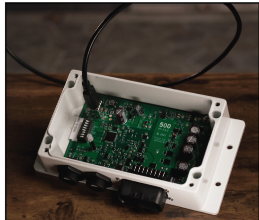
Figure 6 - Type B USB cable connected
