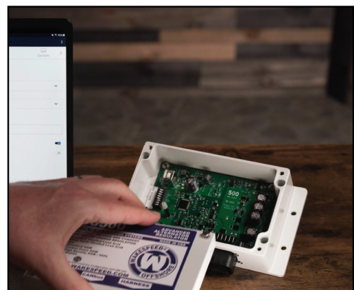
Figure 2 - Removing the regulator lid
