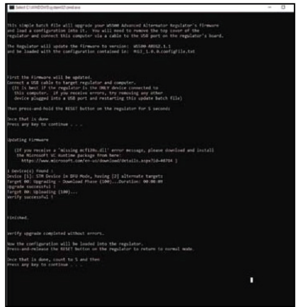
Figure 10 - Batch file window. Showing firmware update.
