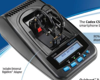
The **Cadex C5100** is a storefront battery analyzer that allows staff to test smartphone batteries from 500 - 5,000mAh with little training.
