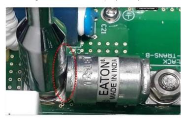
To avoid that fitment issue, use a coupling nut M6x20 (BN), washers (BN), bolts (BN) and spring washers (PBZ) as shown in below photo. These can be supplied by Victron Almere along with the fuses.
