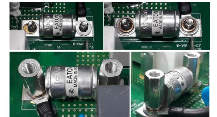
There are two approved fuse PNs of which the brand Vicfuse will not have the fitment constraint due to smaller body size and can be mounted directly on the board with the original nut.
