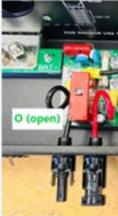
A O (open) grey lever is in down position
