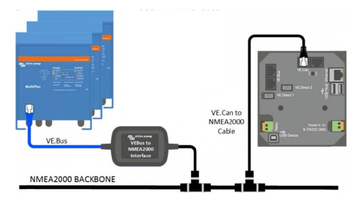
In above example, there needs to be a fuse in the <u>VE.Can to NMEA2000 cable</u>. Without it, the VE.Can port in the CCGX will be left without power and therefore does not work.
