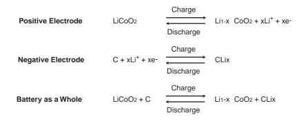
The principle behind the chemical reaction in the lithium ion battery is one where the lithium in the positive electrode lithium cobalt oxide material is ionized during charge, and moves from layer to layer in the negative electrode. During discharge, the ions move to the positive electrode and return to the original compound.
