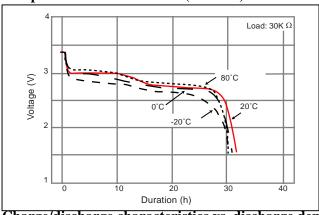
Charge/discharge characteristics vs. discharge depth (VL2020)
