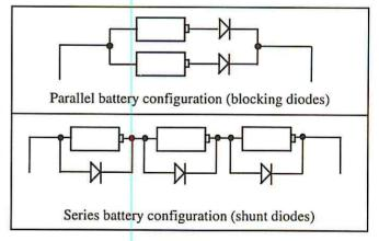
Please remember, this information is provided as general precautions for the use of diodes in lithium battery power supplies. The designer should be aware of other factors that enter into the overall designs of battery packs, including: thermal management, adequate electrical insulation, fusing, and provisions for cell expansion.
