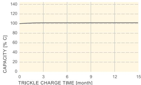
Trickle charge test at +45°C of Ni-MH Button Cells
