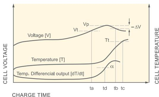
Charging recommended and methods refer to single cells. For batteries there may be different conditions requiring other means of charge or control.
