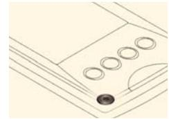
A single VARTA High Rate Cell is used in PDA/Pocket PC to maintain memory content during battery change.
