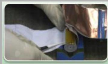
BAJ method: Forced Internal Short-circuit test
