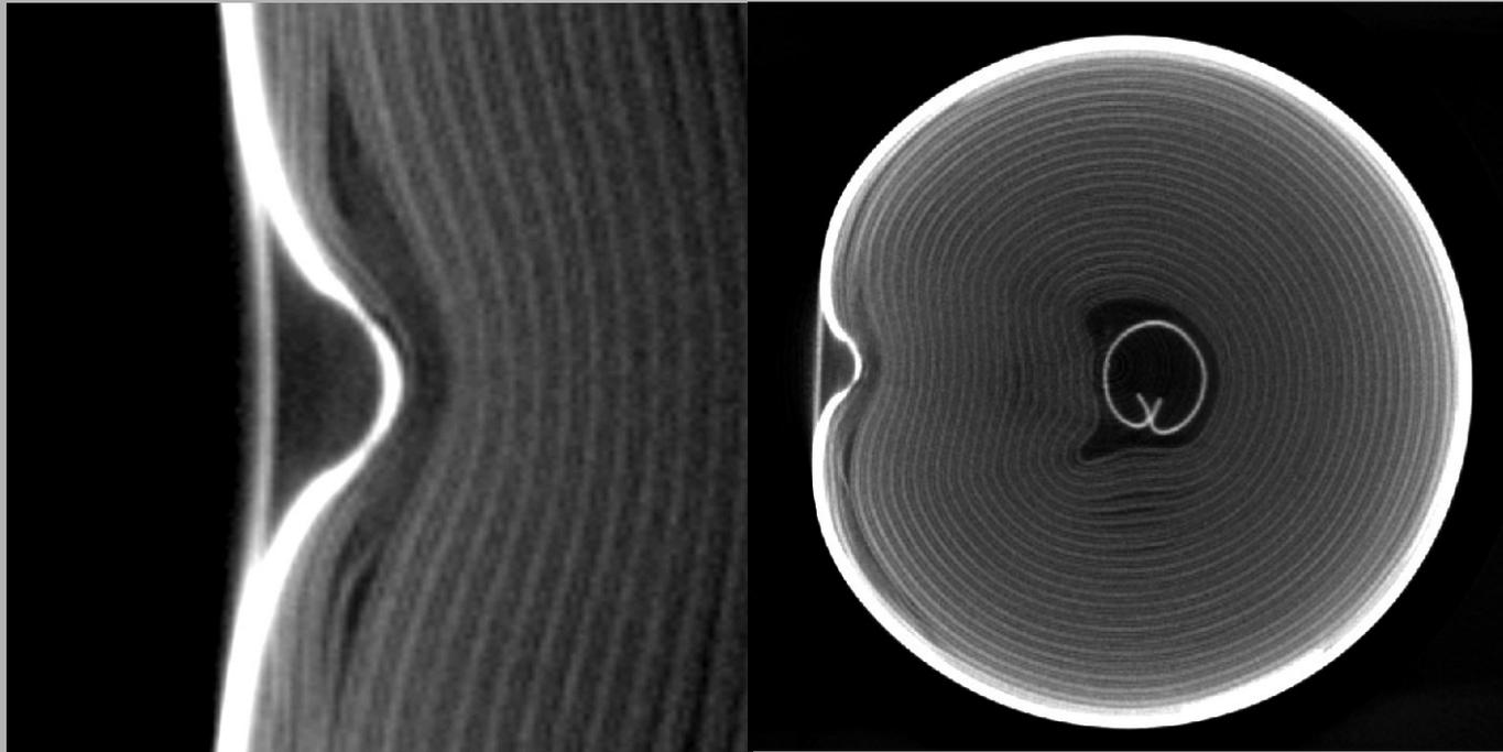
**The CT-Scan of the tested cell shows the short was induced at outer layer/layers.**
