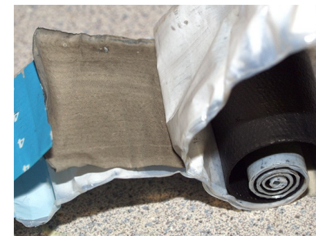
Inside a lithium metal cell
