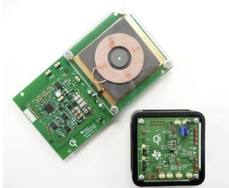
Figure 3: Wireless charging system by Texas Instrument
