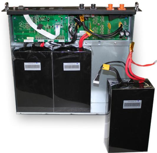
**Example of a system connecting LiFePO4 batteries in series and parallel**
