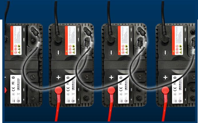
The upshot is that there will be differences in SOC in the batteries throughout most of the cycle life of the battery system. Differences in SOC between batteries means that even when the load is disconnected, there will be eddy current flowing between batteries as they equalise SOC. Eddy currents can be exceptionally high and cause batteries to go into an unpredictable protection mode.
